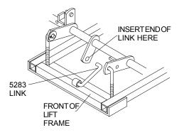
2. Remove front and rear deck hanger pins, as illustrated below.
